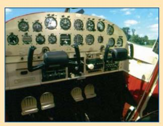
On the floor of the cockpit are pedals that operate the brakes and rudder. When the pilot pushes the right pedal, the rudder turns to the right. It will turn left when the left pedal is pushed.
